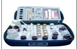
The Jal TARA water testing kit is a portable kit, designed in order to perform the basic tests for ensuring the potability of water and it can be used to assess total 14 parameters which can be divided into 3 broad categories:
